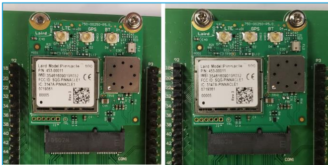
Figure 24: Attaching a 453-00011 Pinnacle™ 100 modem to the Sentrius MG100 Gateway
